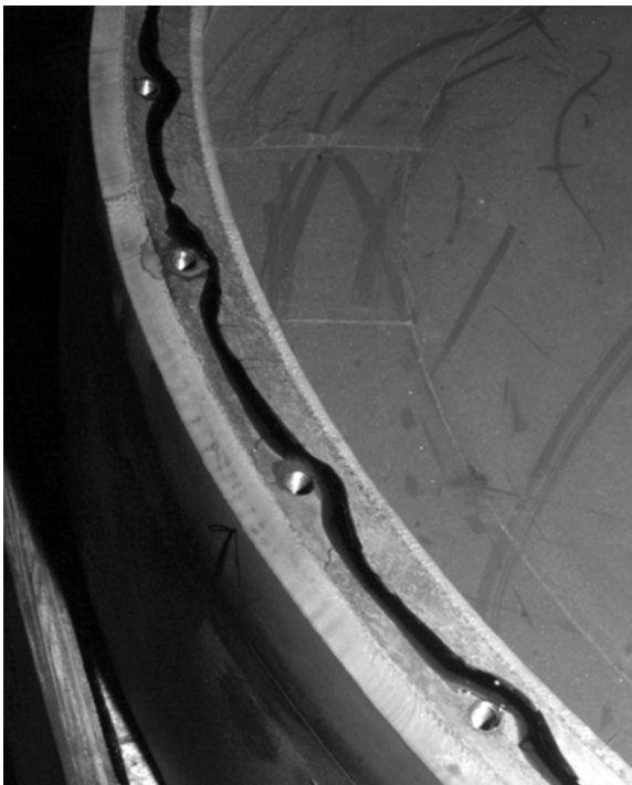
Figure 14: Loctite 515 Applied to Diaphragm Ring
