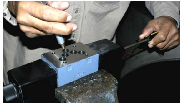
Figure 49: Bench-testing a Directional Valve
