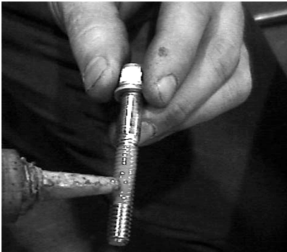
Figure 15: Applying Loctite 242 to Bolts
